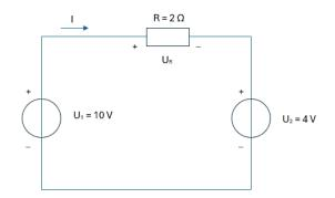
The powers per component can be found by using the formula P=U\*I [W], where the following generally accepted rule applies: where the current arrow I goes in the component, the sign determines that we include in the calculation of the power. That is plus at the resistor R = 2  $\Omega$  and the source U = 4 V and it is a minus at the source U = 10 V. We now get  $P_{10V} = -10*3 = -30 \ W$ ,  $P_R = +6*3 = +18 \ W$  and  $P_{4V} = +4*3 = 12 \ W$ . The sum of the powers is = 0.
